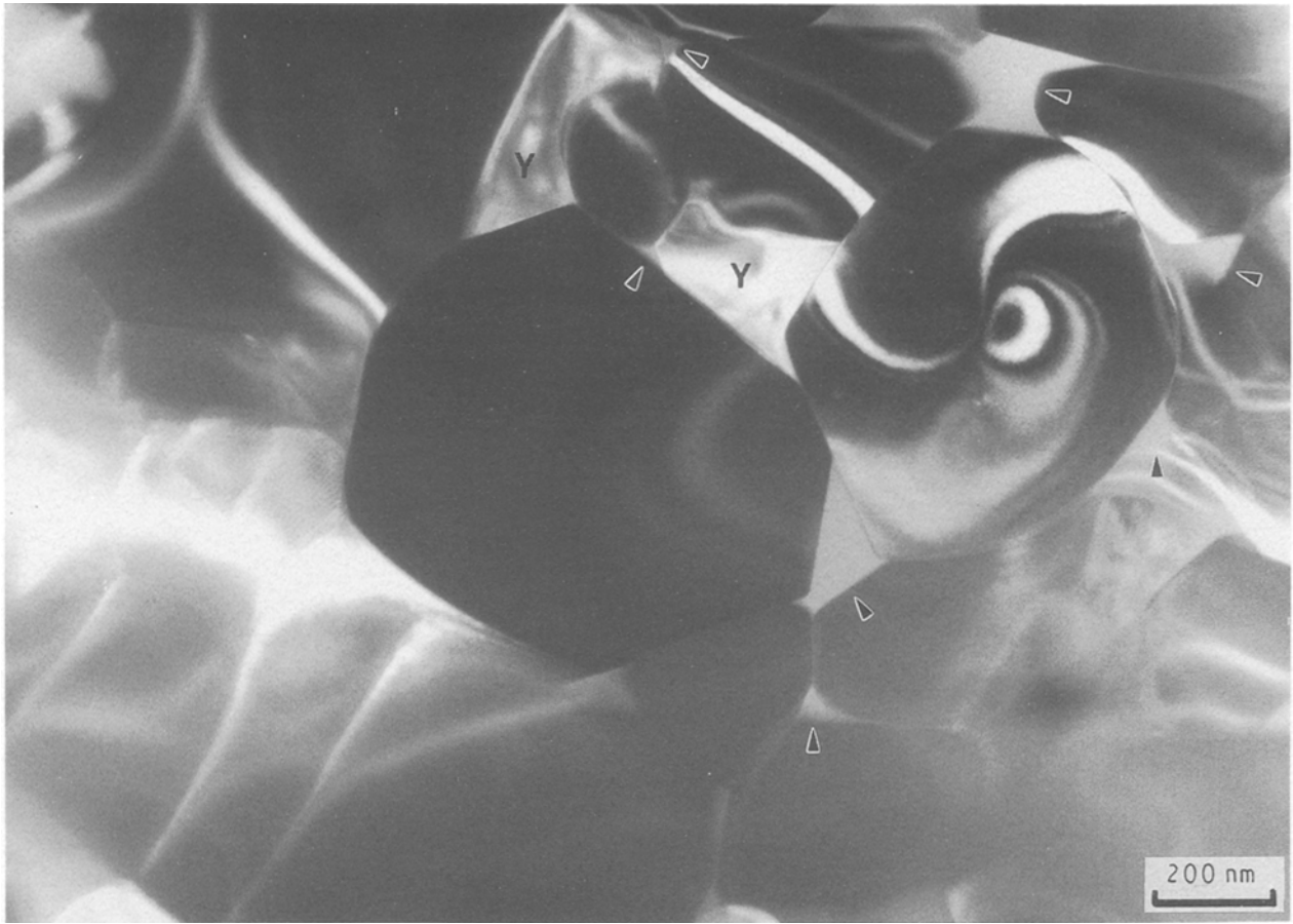
Figure 6 The microstructure of the silicon nitride ceramic after a heat treatment of 20 h consists of residual amorphous grain-boundary phase (arrows), silicon nitride grains and secondary crystalline phase (Y).
